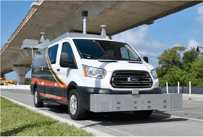
Fig. 14. Example of pavement assessment using IRISpro Pave, similar to the method applied in Beaumont, TX, under ASTM D6433 standards [19].
